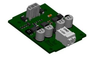
Assignment of connection terminal: 12 V DC (left, viewed from behind - pump upright)
