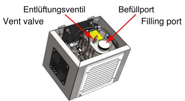
As a second step, the ventilation system of the plant must be enabled and the coolant tank must be filled (*before* starting the pump). To do this, open the top cover of the system with a cabinet key (included).
